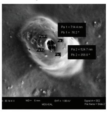
Figure 1. A SEM image of a sub-micron ablation (2 J/ cm<sup>2</sup>, 10 shots) on the surface of a compact disc, chosen as a substrate due to its uniform flatness and organic composition. Although slightly ellipsoid, the ablation is clean with no discernible damage corona. This is vital if small structures such a biological cells are interrogated by laser ablation as peripheral damage can cause structural changes in the yet-to-be-analyzed parts of the cell.
